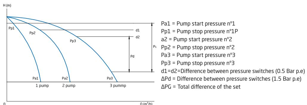
To check the correct operation of the equipment, set the pump selector switches one by one to the "automatic" (AUT) position. Slightly open the valve of the distribution network to check the automatic start and stop pressures of each pump. When this test is completed, close the valve and set all the selector switches on the pumps to the "0" position.
